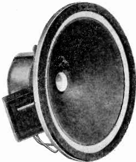
Fig. 9: The white inner ring of this dynamic speaker is made of chamois, and supports the free edge of the cone.
