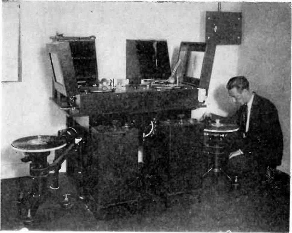
This photo shows the equipment used at station WOR for the broadcasting of recorded programs. A total of four turn-tables is available.
